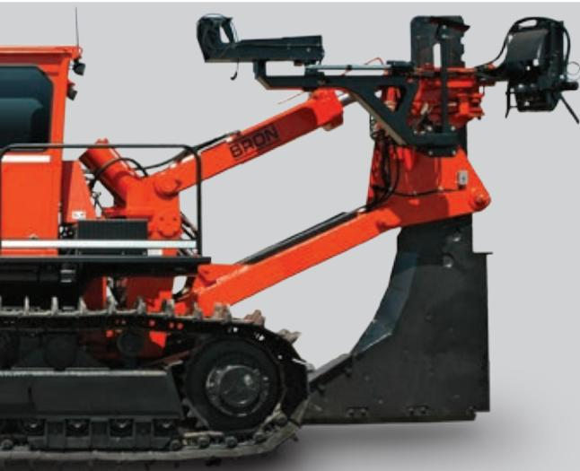
This plow performs best in hard, rocky or soft soils where a regular parallel plow would have difficulty maintaining grade. The 750 RC is a modified parallel plow with total control of both blade and pitch. The blade depth is either GPS or laser controlled, while the blade pitch is controlled by a slope control. Having total blade control and fast responding hydraulics give you a plow for all those tough conditions.
