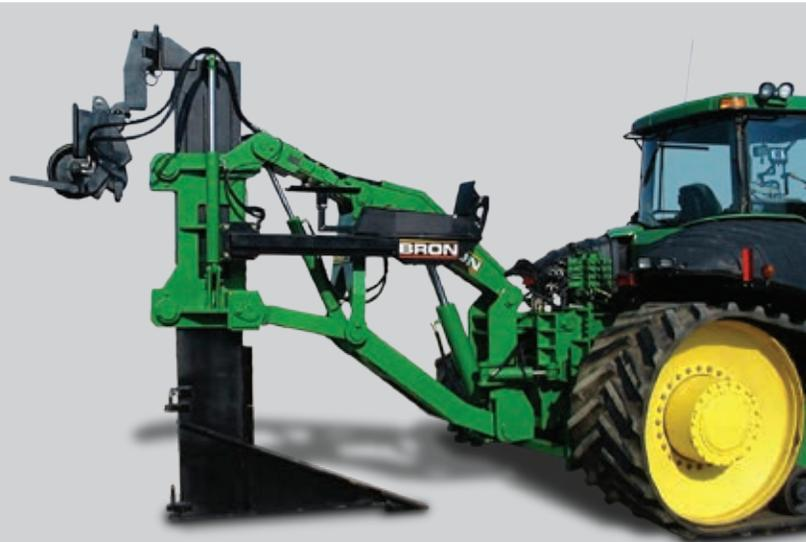
The BRON Add-on Double-Link Plow gets you in the ground as the most economical method of providing accurate tile installation to customers. Available for all sizes of dozers and agricultural tractors, the BRON Add-on Plow has five models for 90-350 HP applications. The quick-attach system makes it easy to disconnect the plow when not in use.
