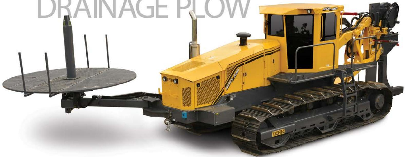
Combining the features of BRON's larger drainage plows with the requirement of lighter road weight comes the BRON 350 Self-Propelled Drainage Plow. Weighing only 58,000 pounds, the 350 offers you BRON technology and design on a D6 undercarriage.
